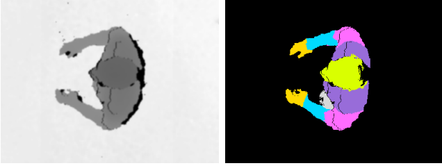
Fig. 4. Left : Depth frame from the real-world ceiling sensor, with a person standing in its' field of vision. Right : Inferred labeling of the depth data, based on point cloud distance heuristics and the sphere representation of the human body.
