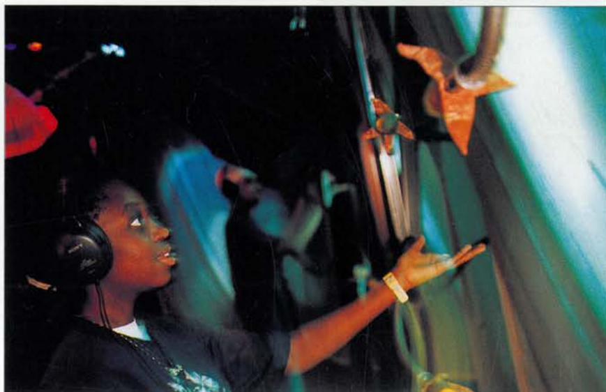
FIG. 5: The Gesture Wall detects your movements with four sensors that resemble flowers mounted on goosenecks at the corners of a large rear-projection screen. (Courtesy MIT Media Lab)
