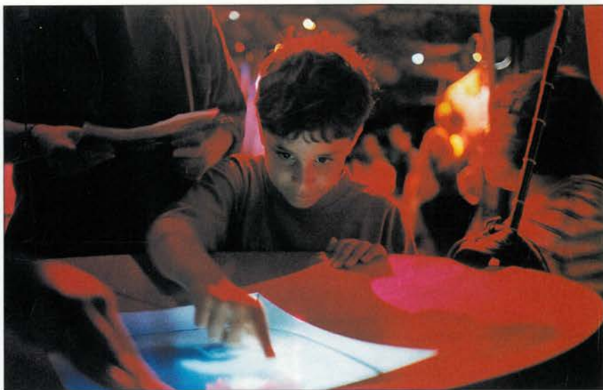
FIG. 3: The Melody Easel lets you “draw” a melody with your finger on a touchscreen. (Courtesy MIT Media Lab)
