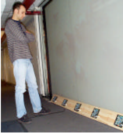
Figure 23: Projection wall with five sonar rangefinders detecting occupants (left) and response of this ensemble to person walking by (right)
