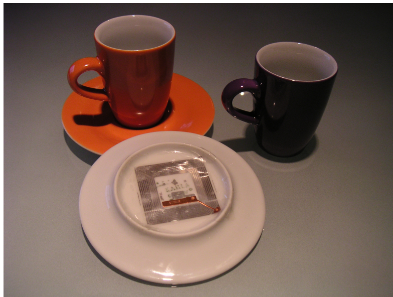
Figure 3.4: RFID transponder attached to underside of saucer.
