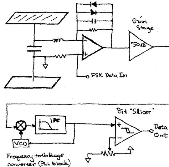
Figure 3: Block diagram of the PAN III transceiver.
