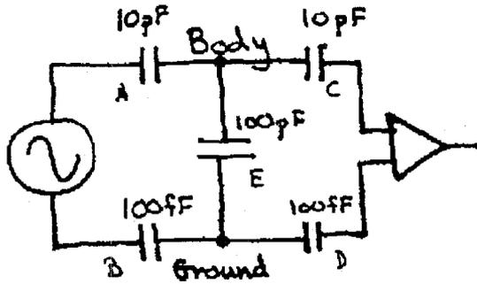
Figure 2: Capacitive bridge formed in Figure 1.
