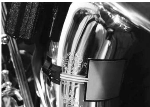
Figure 6. Bell of the Metasaxophone showing the microprocessor casing, the front bell trigger sensor, and the Selmer Insignia.
