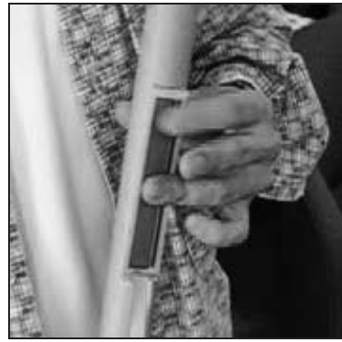
9b. Closeup of linear potentiometer FSR on The Stick.
