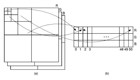
Fig. 2. Procedure used to construct a chromosome. (a) Wavelet transformed  $256 \times 256$  images. (b) The chromosome constructed using the wavelet coefficients of (a).
