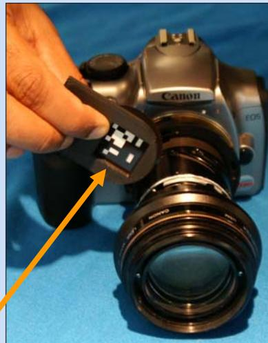
Insert a **coded mask** with chosen binary pattern
