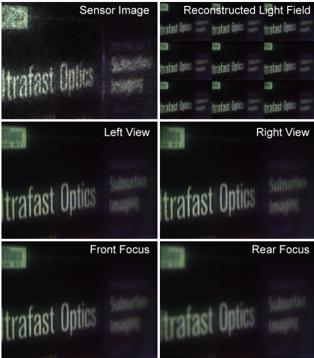
Figure 10: Light field reconstruction from prototype camera. The sensor image (upper left) is optically modulated prior to capture by a random attenuation mask; using the algorithms described in this paper, we reconstruct the light field (upper right). While the individual views of the light field (center row) exhibit slight reconstruction noise, these artifacts are barely visible in the refocused images (lower row).
