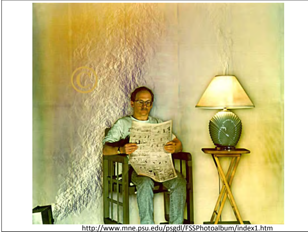
Full-Scale Schlieren Image Reveals The Heat Coming off of a Space Heater, Lamp and Person
