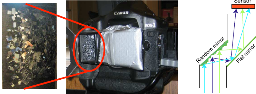
Figure 5: A closeup of the random reflective surface and camera setup used in our experiments. The schematic diagram on the right shows the light path to the sensor.
