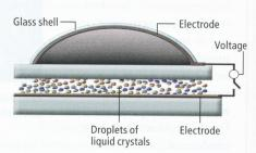
ADAPTIVE LENS uses a convex electrode that produces an electric field whose strength varies from center to edge. The light-refracting liquid crystals respond in kind, enabling changes in focal length (zooming).
