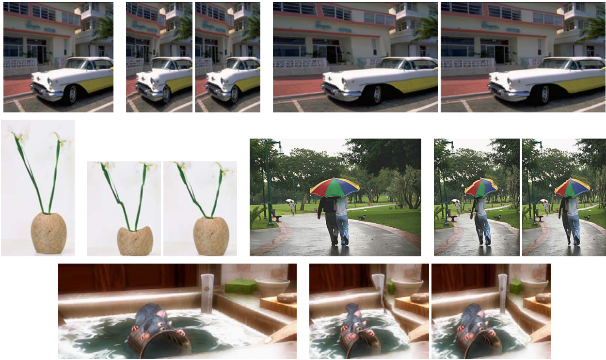
Figure 9: Several comparisons between the original seam carving algorithm (left image of pairs) and forward energy (right image of pairs). At the top the car image (first on the left) was first condensed and then extended. Note how the artifacts on the car and background building are greatly reduced. In the middle, both height and width reductions are shown. At the bottom, one frame from a video resizing is given for comparison. The sequence can be seen in the accompanied video.
