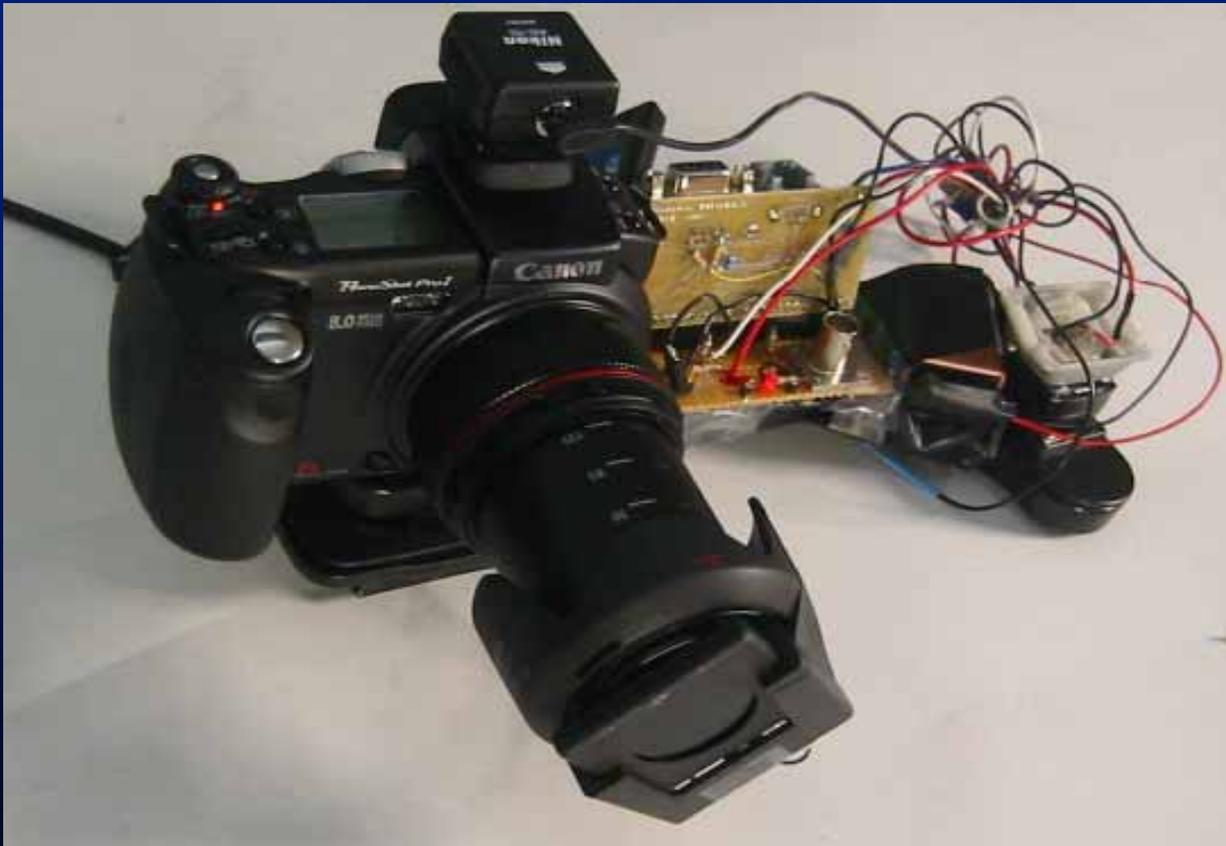
Ferroelectric shutter in front of the lens is turned opaque or transparent in a rapid binary sequence
