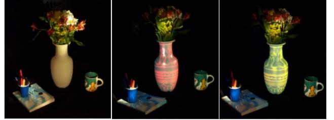
**Figure 4: (Left) The underlying physical object is a white diffuse vase. (Middle and right) View-dependent effects, such as specular highlights, can be generated by tracking the user's location and projecting images on the vase.**
