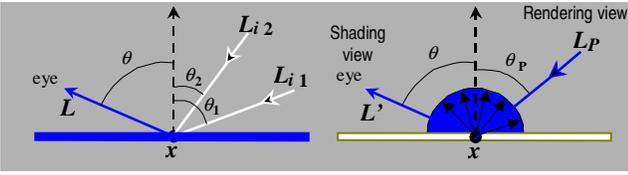
**Figure 3: (Left) The radiance at a point in the direction  $(\theta, \phi)$ . (Right) The radiance as a result of illumination from a projector lamp. By rearranging the parameters in the optical path, the two can be made equal.**
