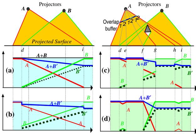
**Figure 6: Intensity weights using feathering methods. The plots show the contribution of projectors  $A$ ,  $B$  and  $B'$  and the resultant accumulation  $A+B$  and  $A+B'$  along the lit planar surface. Our technique, shown in (d), creates smooth weight transitions.**
