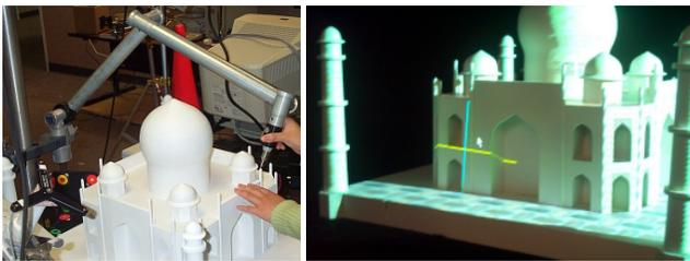
**Figure 8: (Left) We use a 3D touch probe scanner to create a 3D model of the real object. (Right) The projectors are calibrated with respect to the model by finding which pixels (center of cross) illuminate the known 3D fiducials.**
