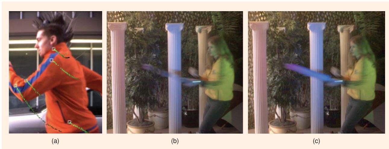
FIGURE 1 A new high-speed optical motion capture system [4], developed at Mitsubishi Electronic Research Laboratories (MERL), can measure 3-D motion, orientation, and incident illumination at tagged points in a scene. (Photo courtesy of Ramesh Raskar of MERL.)
