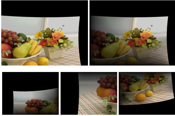
Figure 3: Top row: Image in top-right projector’s framebuffer, before and after attenuation with alpha map \Phi_i . Bottom row: Other three projectors with intensity correction. Note the outer black areas which are automatically generated after quadric transfer.
