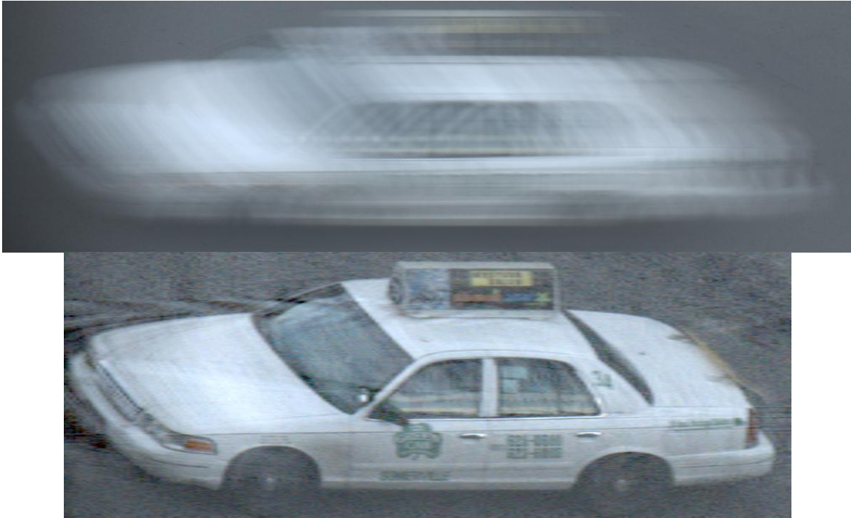
Figure 10 Preserving High Spatial Frequencies using a Flutter Shutter Camera. (Top) Photo of a fast moving taxi taken with coded exposure camera. Notice the subtle patterns in the blur which appear as multiple replicas rather than a continuous smear. (Bottom) The deblurred image. (Raskar et. al. 2006)
