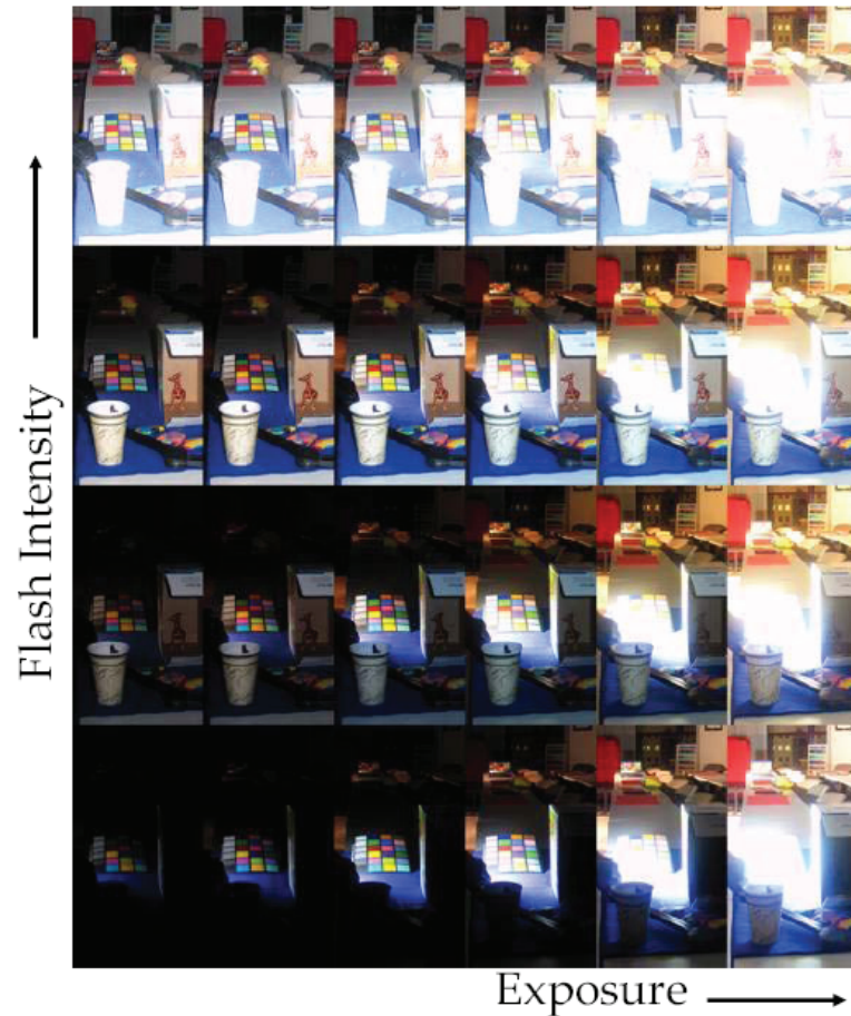
Figure 4.4. Flash exposure high dynamic range sampling [Agrawal et al. 05]
