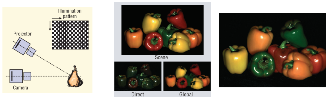
Figure 4.10. The projector can be used as a programmable camera flash. By projecting high frequency (checkerboard) patterns, one can separate direct and global illumination effects.
