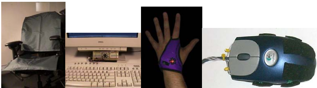
Figure 1: Various sensors can capture postural, facial, skin-surface, and gestural changes that carry affective information. From left to right: Chair with Tekscan pressure sensors, BlueEyes camera, Galvactivator skin conductivity sensor, and Pressure Mouse.
