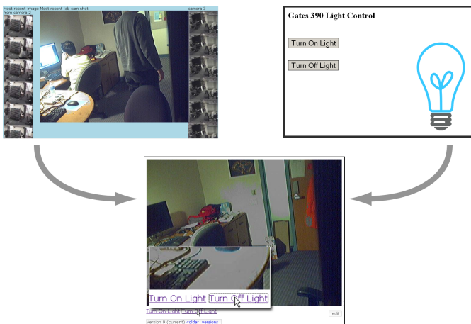
Figure 5. An example of a d.mix ubicomp mashup: web services provide video monitoring and lighting control.
