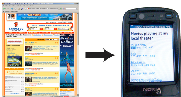
Figure 4. The rewriting technology in d.mix can be used to tailor content to mobile devices. Here, essential information is extracted from a movie listings page.
