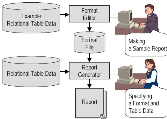
**Figure 2 System Configuration**
