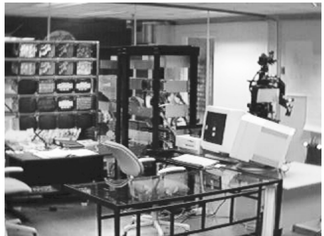
Figure 2: Cog is the humanoid robot used in our experiments, shown on the right. The “brains” of cog is a MIMD computer shown in the center of this image. The contents of DPRAMs (images, processed images, maps, etc.) can be displayed on a bank of twenty displays shown on the left. The Macintosh Quadra is the front end to the MIMD computer.
