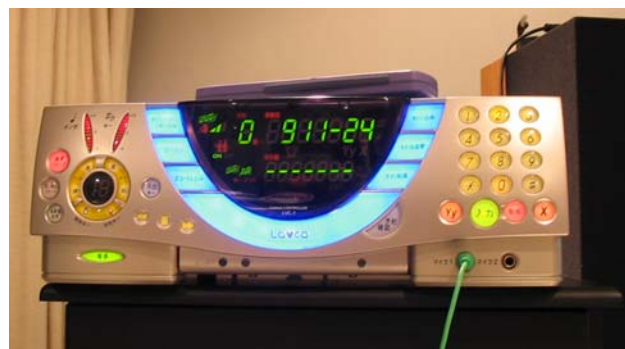
Fig 5 Taito Corporation's Lavca System, the audio industry's first professional audio product based entirely on software audio processing. Using Multiprocessor Csound running on 3 SIMD dual-core floating-point DSPs from Analog Devices, the system delivers 64 voices of MIDI synthesis, real-time tempo-varying MPEG decode, tempo-following voice-tracking, and comprehensive audio-post-effects processing, all at 48 kHz in 2- or 4-channel sound. Each system contains 40 000 songs, outputs high-quality graphics and synchronised text, and has a unique IP address for updating in the field.
