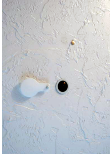
(a) View of the ceiling showing the camera, open privacy shutter, and boundary layer microphone. (b) HP iPaq with recording and control software.
