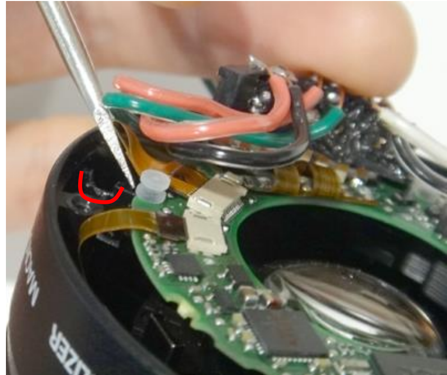
A few wires can be laid through this gap
