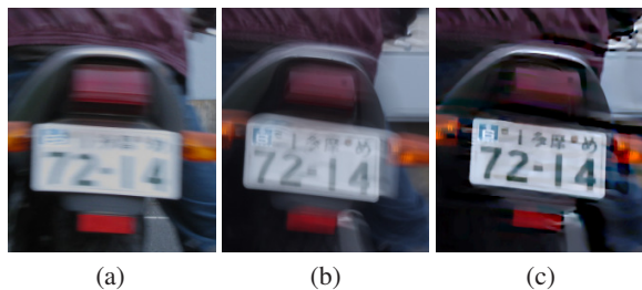
Figure 20: License plate of a motorbike. (a) From a static camera. (b) From the circular motion camera. (c) Deblurring result of (b).
