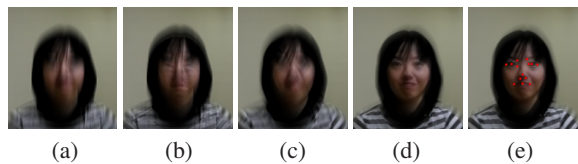
Figure 21: Motion-blurred face simulated from high speed camera images. (a) Static camera. (b) Coded exposure camera. (c) Motion-invariant camera. (d) Circular motion camera. (e) Facial feature point detection succeeded for the circular motion camera image (d) without deconvolution (and failed for the others (a-c)).
