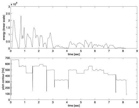
**Fig. 15.** Synthesis (loop of the 16-note excerpt): energy envelope and pitch contour of an expressive morphing. The expressive intention changes smoothly from heavy to soft. The final rendering is the result of the audio transformations controlled by the model and performed on the neutral performance.
