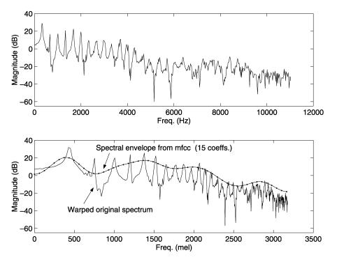
**Fig. 7.** Spectral envelope representation by mel-cepstrum coefficients. Upper panel: original spectrum (frequency axis in hertz). Lower panel: warped and smoothed version of the original spectrum, and the spectral envelope obtained by using 15 mel-cepstrum coefficients (frequency axis in mel).
