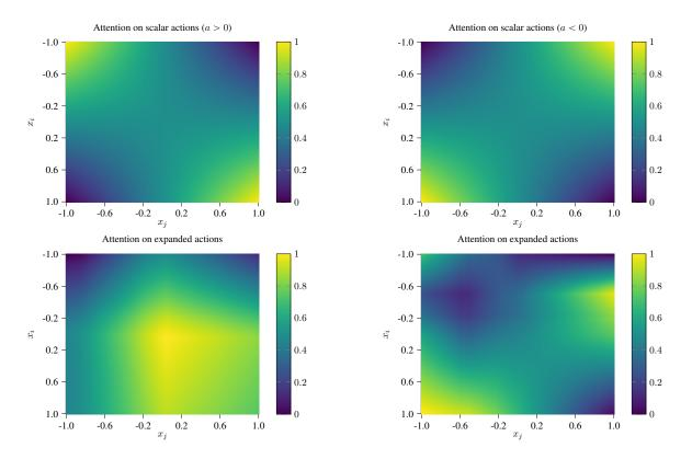
Figure 12. Top, attention values for a multiplicative attention layer directly operating on the input scalars  $x_i \in [-1, 1]$ ,  $x_j \in [-1, 1]$  with positive (left) and negative (right) coefficient. Bottom, attention values for a multiplicative attention layer with random coefficients processing the expanded actions  $y_i$ ,  $y_j$  of  $x_i$ ,  $x_j$ . The result is scaled to [0, 1] for visualisation purposes.
