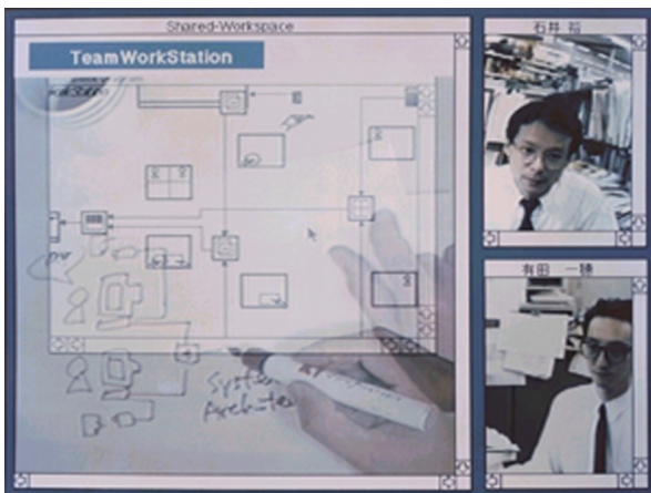
TeamWorkStation interface with half-transparent overlays of workspaces on the left and video of collaborators on the right
