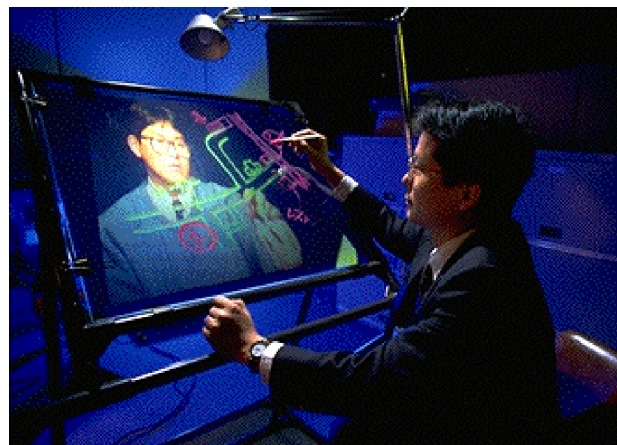
ClearBoard interface with shared drawing space and implied face to face interpersonal space between two collaborators
