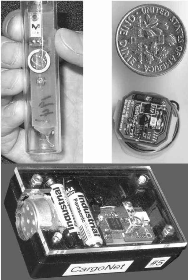
Fig. 16.5 An ultra low-cost wireless motion sensor for crowd interaction (top left), quasi-passive optical wakeup tag (top right), and a CargoNet Active RFID Sensor Tag (bottom)
