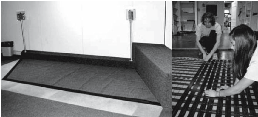
Fig. 16.3 The Magic Carpet Installation at the Boston Museum of Science (left) and taping of the piezoelectric wire to the bottom of the carpet (right) before installation at the MIT Museum
