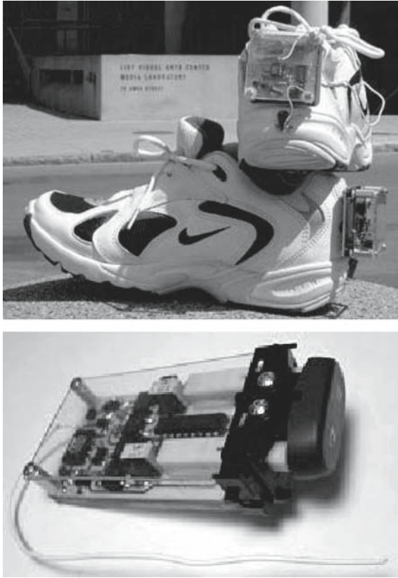
Fig. 16.7 Power generating shoes with piezoelectric insoles from 1998 (top) and a self-powered dual RF push button for a wireless car window controller (bottom)
