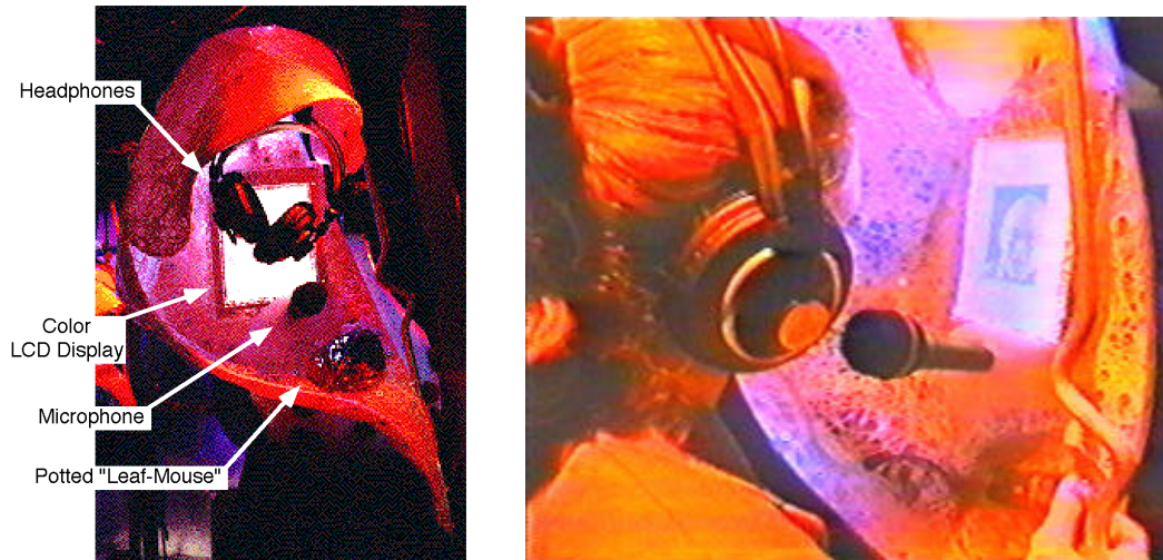
Figure 3: Layout and photograph of a Speaking Tree
