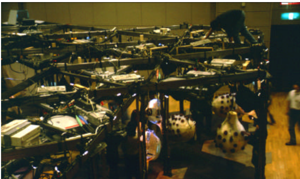
Figure 1: Overhead view of the Brain Opera Lobby truss structure, as being assembled before a Tokyo run in November 1996. All electronics are mounted atop the truss, leaving only the interactive interfaces (such as the Rhythm Tree bags at lower right) visible to the participants
