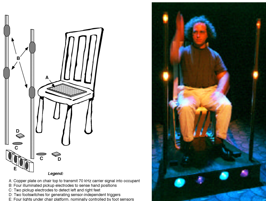
Figure 15: The Brain Opera's Sensor Chair; diagram (left) and in performance (right)
