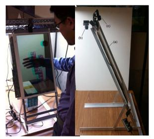
Figure 2. User is interacting with virtual content by reaching behind display. Figure 3. System side view: (a) transparent LCD panel; (b) depth camera; (c) Webcam.
