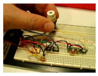
On the lower left side is the PIC visible (UV erasable), on the right side the Radiometrix transmitter. I am holding the compass. This configuration was for debugging; eventually, all components will be replaced by surface mount equivalents and soldered directly to each other.
