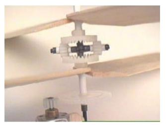
Coax counter rotating rotors by Kai Huber. The rotor airfoil design is not very sophisticated, e.g., not taking in account downwash from upper rotor. The pitch angle and probably the airfoil itself should be different for the upper and lower rotor.
