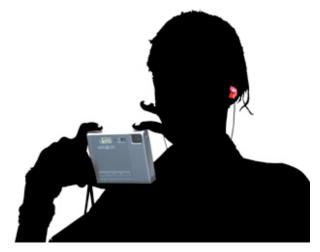
Figure 1: Depiction of the RAW tool, with digital camera and ear-microphones for binaural audio recording.
