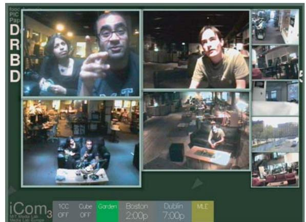
The system conserves bandwidth by reducing frame rate where no activity is detected and by not transmitting audio when nobody is speaking. Clicking the windows changes their arrangement, allowing the display to be customized for a particular activity. Transmitted resolution is adjusted to reflect the size of the window. Use of connectionless networking protocols enables the system to operate effectively in congested or problematic networks.
