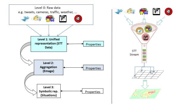
Figure 6.1: The workflow of data from raw streams to situation descriptors
