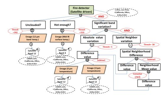
Figure 9.18: 'Wildfire' recognition model using satellite data
