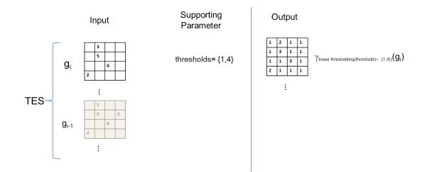
Figure 6.7: Example: Classification operation based on linear thresholding pixels have been assigned. The class assignment corresponds to the thresholds set.
