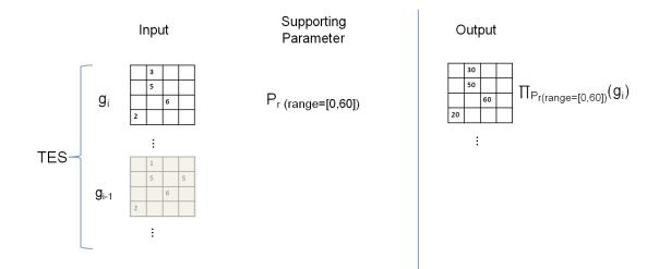
Figure 6.5: Example: Filtering operation to normalize values to a range mapped from an initial range of 0 to 6, to the new range of 0 to 60.
