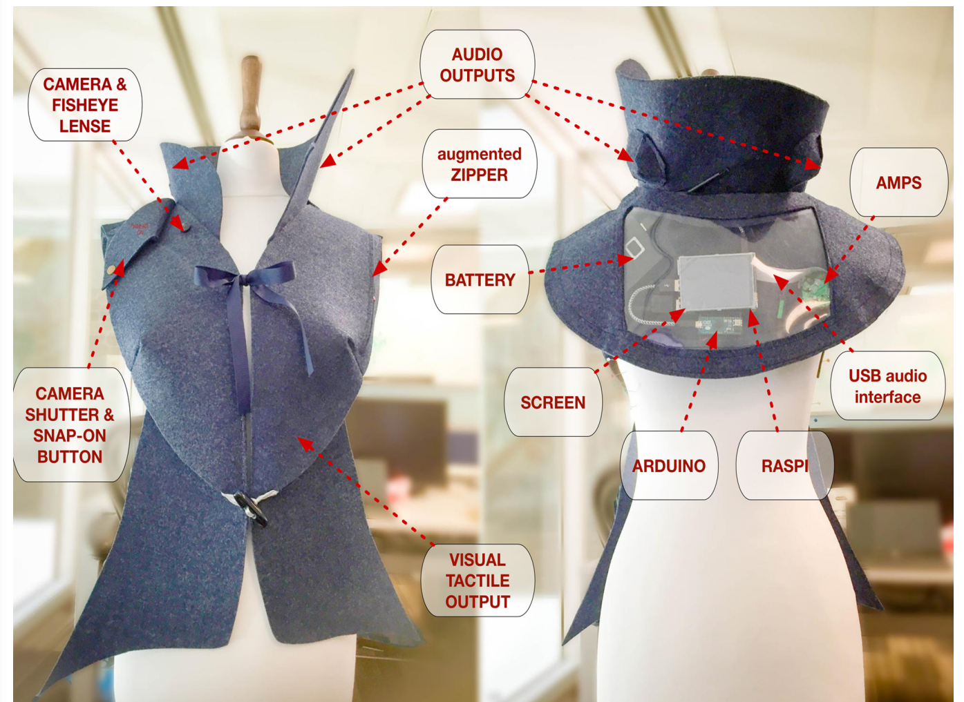
Figure 7. The SNaSi garment and its hardware components. The input sensors are a fisheye camera and zipper potentiometers, the main output is the 3D audio speaker system (amplifiers and voice coils) contained in the collar. The longer parts on the front were originally designed to possibly support a visual-tactile display but it not present in the current prototype.
