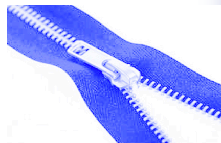
Figure 9. By sewing conductive thread along the two sides of a regular metal zipper we created a zippotentiometer capable of sensing the precise percentage of opening/closing of the zipper. When added to the garment, it allows the user to have continuous control of the system.
