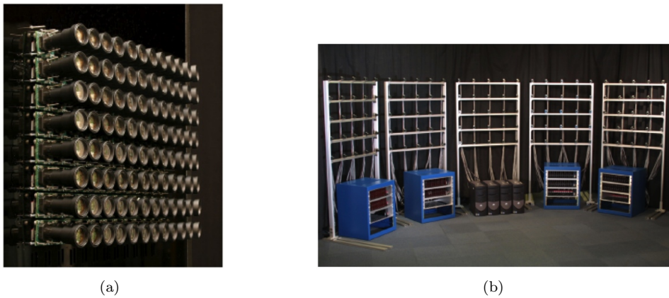
Figure 3.3: Camera array setups from Stanford University can capture multiple photos simultaneously from slightly different viewpoints for epsilon changes in parameters over sensors. (Figures from Wilburn et al. [427].)
