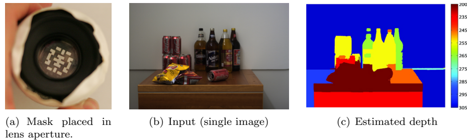
Figure 4.22: Depth estimates from a conventional camera with a coded aperture. (Figure from Levin [231])
