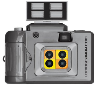
Figure 3.7: The Lomography Actionsampler Flash 35mm film camera uses multiple flashes and four lenses to capture multiple photos in quick succession. Each photo is taken from a slightly different point of view, and at a slightly different time.
