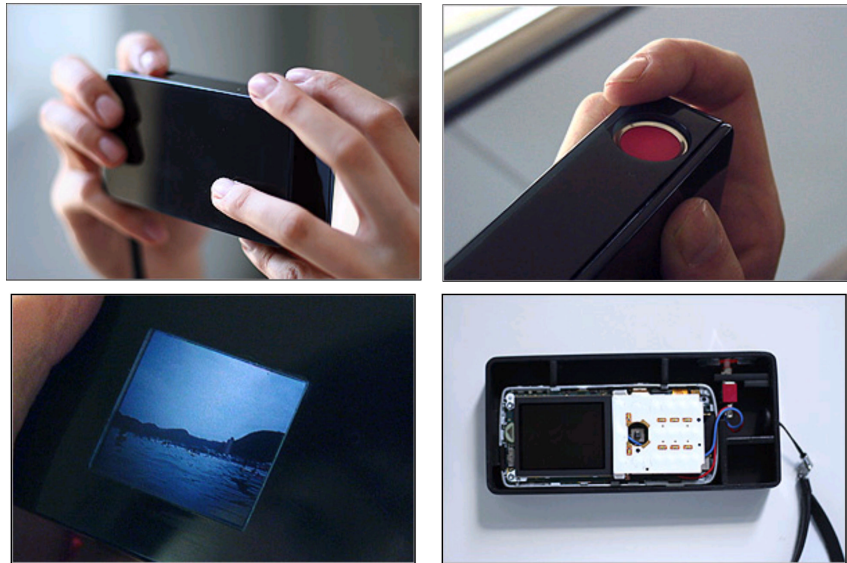
Figure 8.8: The Blind Camera has no traditional camera optics. When you take a picture, the camera connects to the internet, searches for photos from the same location with a similar time stamp, and returns a picture to the viewfinder display.
