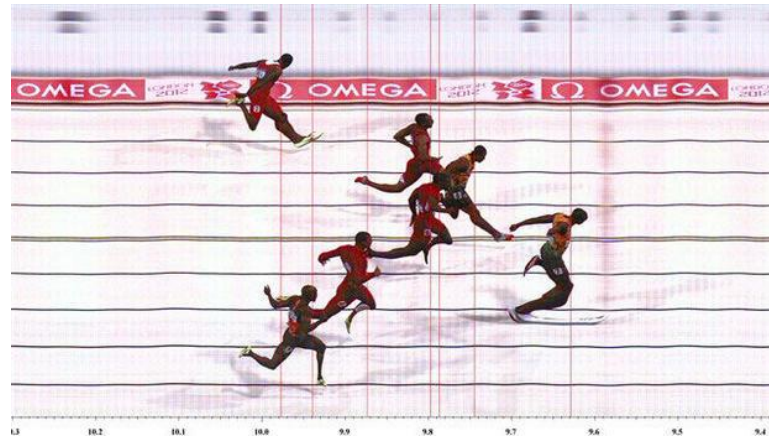
Figure 6.2: The line scan camera takes an image whose horizontal axis measures time instead of position.
