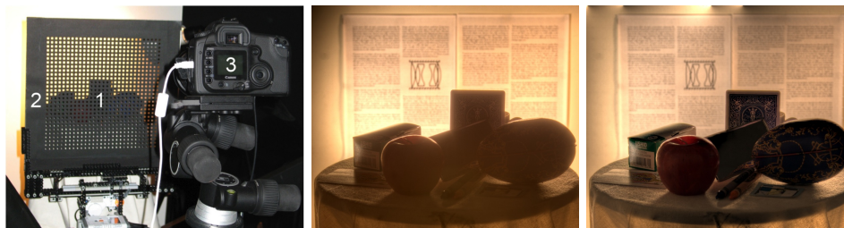
Figure 4.19: (left) Setup used by Talvala et al. [389] for glare reduction. (center) Glare reduces the contrast in the photo of a scene with backlight; (Right) Glare reduced and contrast increased using the technique described in the paper. (Figure from Talvala et al. [389])
