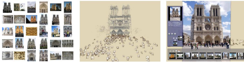
Figure 7.21: Photo Tourism: Exploring Photo Collections in 3D [376]. (Left): An input collection of unstructured photographs of a single scene found by on-line image search. (Center): Structure-from-motion on corresponding points from all pairs of photos in the collection creates a sparse 3D point-cloud of the scene, along with automatic camera viewpoint recovery for each photo. (Right): Interactive 3D image browsing permits users to navigate smoothly among photos by indicating a desired viewpoint or selecting a portion of the 3D point cloud, providing the impression of freedom of movement to tour and explore the scene in 3D. (source: phototour.cs.washington.edu/Photo_Tourism.pdf )
