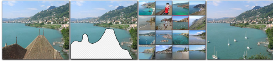
Figure 7.22: Examples from “Scene completion using millions of photographs” [178]. (Far left): The input image and (Middle left): marked region we wish to replace. (Middle right): Searching a large on-line image collection finds several closely-related scenes, (Far right): Use graph-cuts to find suitable boundaries for replacement regions in the source and destination photos, and then combine the pieces using Poisson editing methods to blend them without visible seams. (source: graphics.cs.cmu.edu/projects/scene-completion/ )
