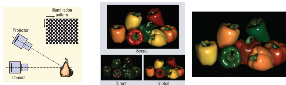
Figure 5.16: Fast separation of direct and global illumination using high-frequency projected patterns. (left) The projector is used as a programmable camera flash. A sequence of shifted high-frequency checkerboard patterns illuminates the scene. (middle) Direct and global illumination components can be easily extracted from the shifted checkerboard sequence. (right) Altering the colors of the peppers in the global component image allows novel image synthesis.
