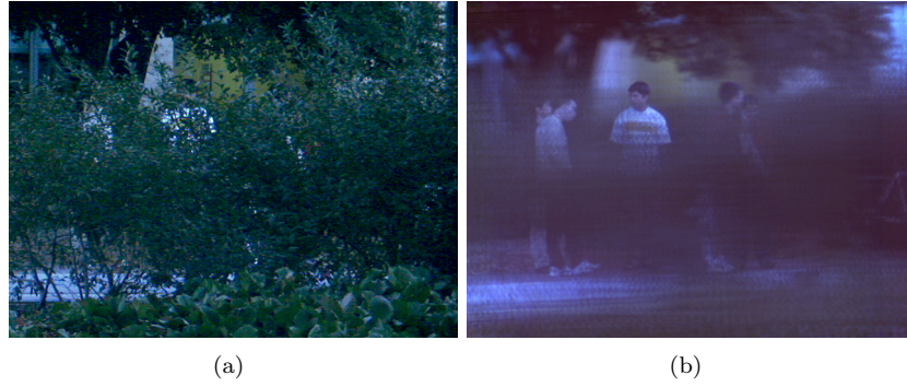
Figure 4.29: Synthetic aperture using camera arrays. (a) Photo from a single camera. (b) Image obtained by combining photos from each individual camera in the array. (Figure from Vaish [410])
