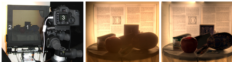
Figure 4.40: (left) Setup used by Talvala et al. [389] for glare reduction. (center) Glare reduces the contrast in the photo of a scene with backlight. (right) Glare reduced and contrast increased by using the technique described in the paper. (Figure from Talvala et al. [389])
