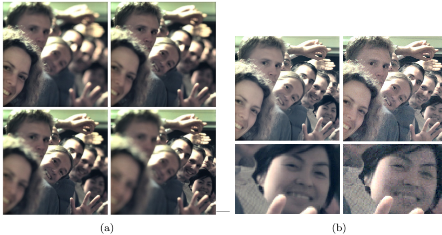
Figure 4.8: (a) Refocusing example from the Stanford plenoptic camera. (b) An all-in-focus image created from the focal stack produced by the light field data has less noise than an image captured by a smaller aperture size to get the same depth of field. (Figure from Ng [303])
