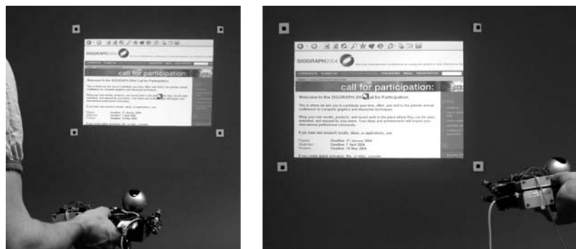
Figure 8.8. Absolute stabilization projects to a fixed location, regardless of projector position. (Images reprinted from [159] © ACM.)
