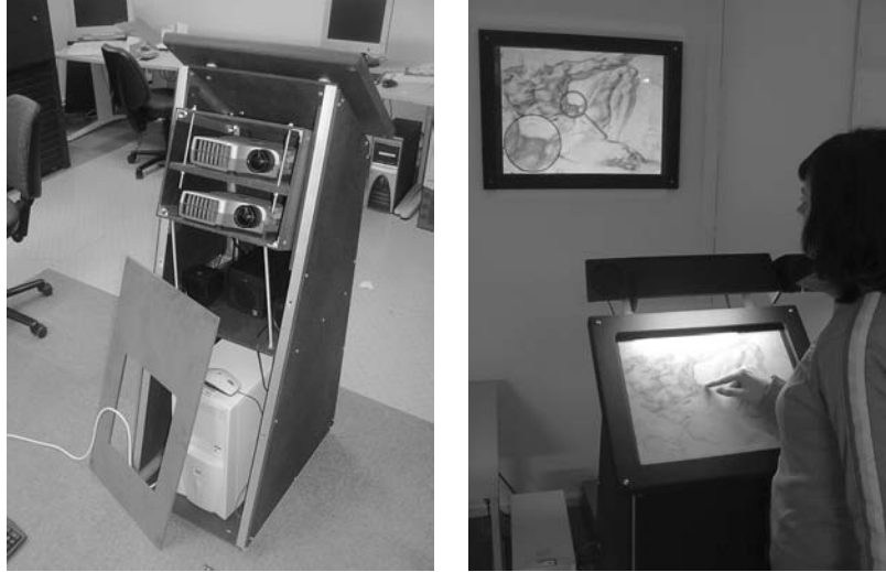
Figure 8.22. Lectern-like display configuration with integrated video-beamers; PC, and touchpad. (Right image reprinted from [19] © IEEE.)
