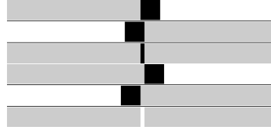
Figure 4.9. Choice (a): Contribution from a single projector at every point in overlap. Top three rows show result of misregistration in case of projectors moving away from each other. Top row, projector moves to left. Second row, projector moves to right. Third row, resulting addition shows a dark gap. Bottom three rows show extra overlap results in a spiked region that is twice as bright.
