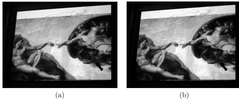
Figure 7.24. Results of color correction process with two projectors: (a) the limited intensity capabilities of a single projector result in visible artifacts; (b) the contribution of a second projector reduces these effects. (Displayed artwork courtesy of the Vatican Museum, Rome and the British Museum, London; images reprinted from [19] © IEEE; see Plate VI.)
