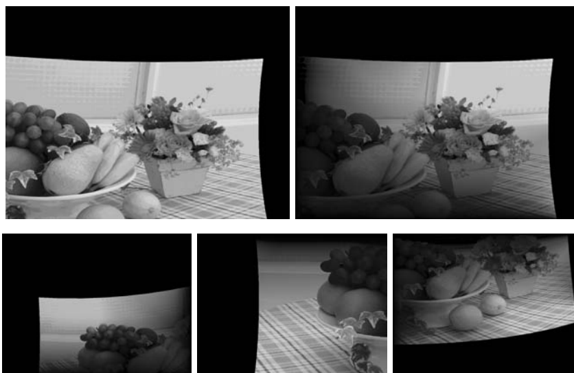
Figure 5.15. Top row: image in top-right projector's frame buffer, before and after attenuation with alpha map \Phi_i ; Bottom row: Three other projectors with intensity correction. Note the outer black areas which are automatically generated after quadric transfer. (Images reprinted from [158] © ACM.)
