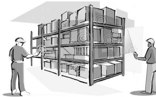
Figure 9.2. Warehouse scenario with RFIG tags. A user directs a hand-held projector at tagged inventory, with communication mediated by two channels—RF and photo-sensing on the tags. The user sees a projection of the retrieved tag information collocated with the physical objects and performs a desktop-like interaction with the projection. A second user performs similar operations, without conflict in the interaction because the projector beams do not overlap. (Image reprinted from [159] © ACM.)
