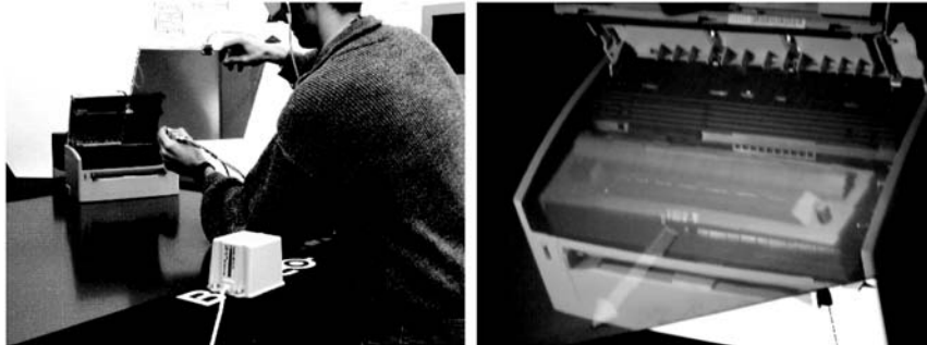
Figure 3.9. The Transflective Pad—a hand-held mirror beam combiner in combination with a large rear-projection screen. ( Image reprinted from [8] © Blackwell. )
