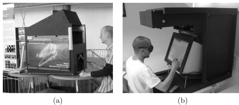
Figure 8.17. HoloStation prototypes: (a) autostereoscopic version with head-finder and force-feedback; (b) active stereoscopic version with infrared tracking and touch-screen interaction; the video beamers are not visible from the outside.
