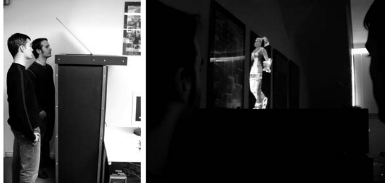
Figure 2.30. First prototype of an autostereoscopic, multi-user capable optical see-through display implemented by the Bauhaus University-Weimar.
