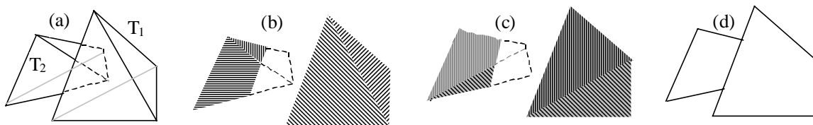
Figure 1. The first layer, P1 , for scene (a) is made up of parts of nearest front facing polygons (b). The second layer, P2 , is made up of parts of back facing polygons (c). The intersection of these two layers in image space creates silhouette edges (d).
