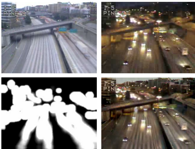
Figure 9: Enhancing traffic video. (Top row) A high quality daytime and a low quality nighttime image, (Bottom row) The importance image obtained after processing, and the final output of our algorithm. Notice the road features and background buildings (Video available at project website).
