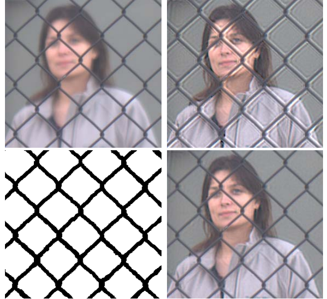
Figure 13: Deblurring in presence of partial occluders. (Top Left) Blurred photo of a person occluded by the in-focus fence. (Top Right) Deblurring without taking the occluders into account results in artifacts. (Bottom Left) Binary mask for the occluders. (Bottom Right) By solving the weighted deconvolution equation, one can remove these artifacts.
