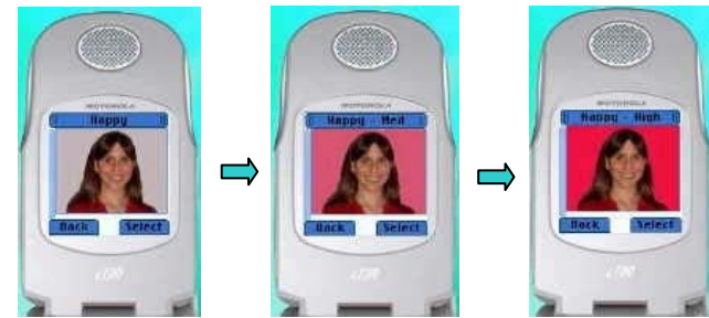
Figure 4: The progression of screens shown when someone is happy and exhibits high arousal, as measured by the galvactivator glove.
