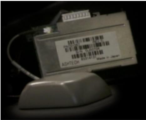
1. A differential GPS unit – Ashtech SK-8. GPS stands for Global Positioning System, a satellite-based system used to deliver real-time position of GPS clients. The SK-8 consists of the main unit (1.57x2.44x0.47 inch, 0.7oz), and a 1” antenna. The unit picks up the satellite signal, deciphers it and passes it to the wearable’s CPU (CutBrain). *The SK-8 GPS* is differential ready, a feature allowing it to provide much better precision in determining user’s coordinates (precision = 2→5 meters).
