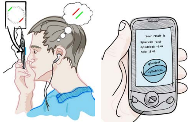
Figure 1: Can a person look at a portable display, click on a few buttons and recover his refractive fidelity? Our solution combines inexpensive optical elements, programmable display and interactive software components to create the equivalent of a parallax barrier display that interfaces with the human eye. Using this platform, we create a new range of interactivity for measuring several parameters of the human eye, such as refractive errors, focal range, and focusing speed.
