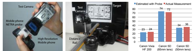
Figure 12: Our probe is used to test refocusing speed (left) and focus range (center). Closest distance at which different camera-lens configurations can focus at (right). The blue bars are estimated distances with our probe. The red bars are estimates obtained using an optical bench.
