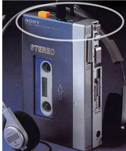
Figure 5. Sony's original TPS-L2 Walkman, with dual headphone jacks, microphone, and an orange button for allowing two listeners to communicate with each other. (13, 2004)
