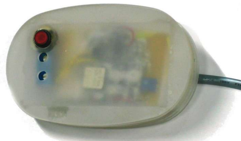
Figure 4. Limor Fried's "Wave Bubble" jams cellular telephone signals in a bubble around its user. Also, instructions to build it are available online. (12, 2005)
