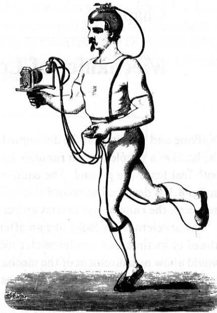
Figure 3.1: Marey's instrumented runner
