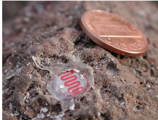
Figure 4.7 Light Sensor Embedded in Fake Rock
